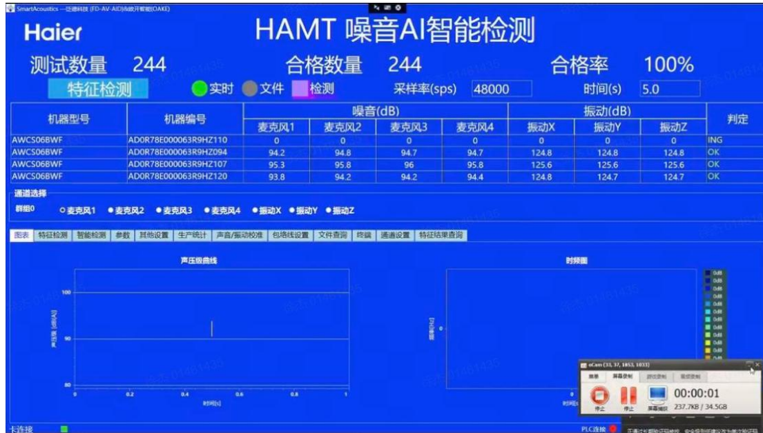
Figure 3: AI Online Inspection System
