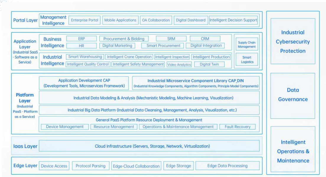
Figure 1: Huaxin Building Materials Smart Factory Overall Architecture Diagram
