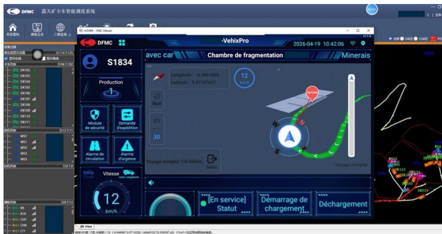
Figure 3: Intelligent Truck Dispatching System of the Simandou BWCS Intelligent Mine
